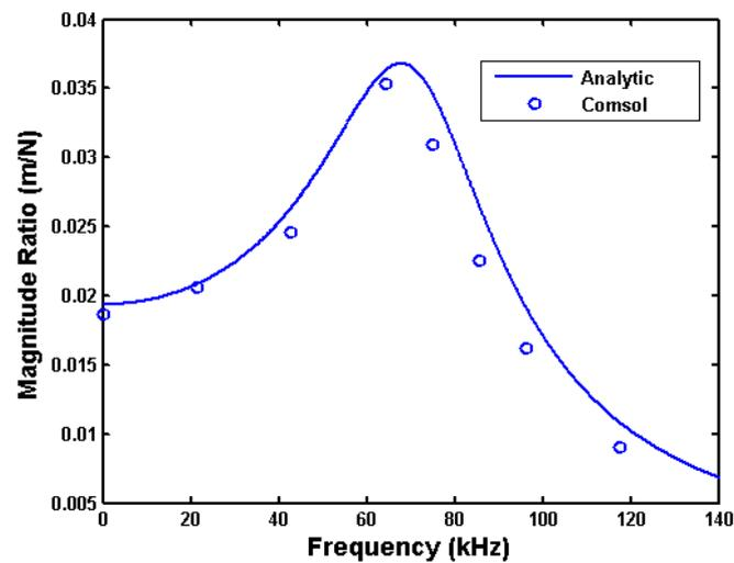
**Figure 6.** Comparison of analytical and numerical frequency responses for square plate with  $67\ \mu\text{m} \times 67\ \mu\text{m}$  hole, at ambient pressure of 300 Pa, with folded leg stiffness of 51.65 N/m.
