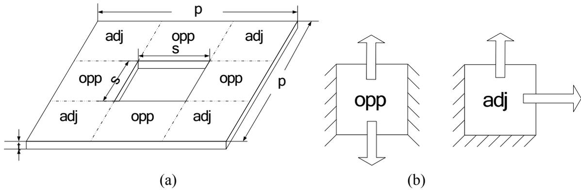
According to Darling’s model [14], the spring and damping constants, respectively, for a plate with two opposite edges venting are:
