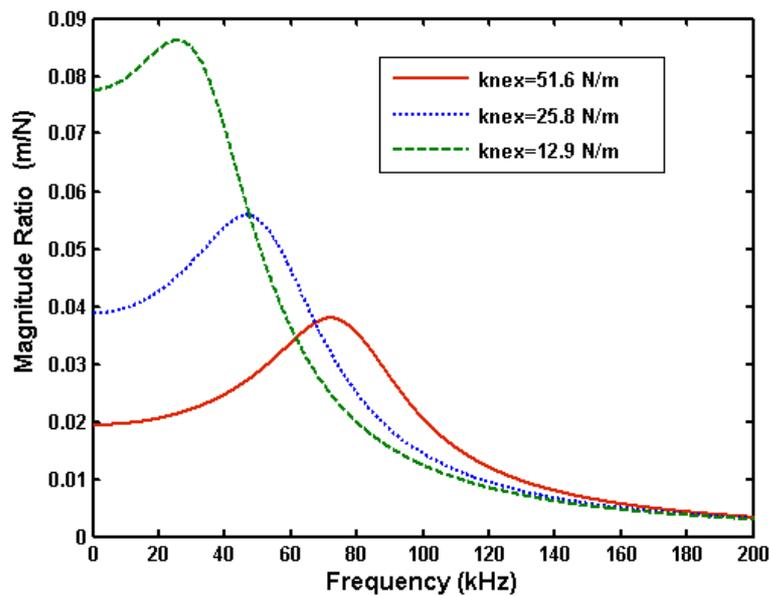
**Figure 4.** Effect of hole size on frequency response of square plate resonator with leg stiffness of 51.6 N/m and 3,000 Pa ambient pressure.
