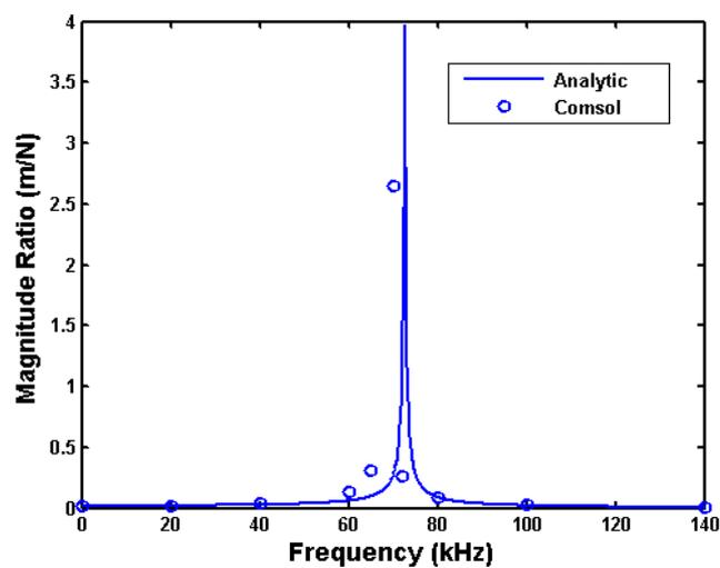
**Figure 7.** Comparison of analytical and numerical frequency responses for square plate with  $5\ \mu\text{m} \times 5\ \mu\text{m}$  hole, at ambient pressure of 300 Pa, with folded leg stiffness of 51.65 N/m.
