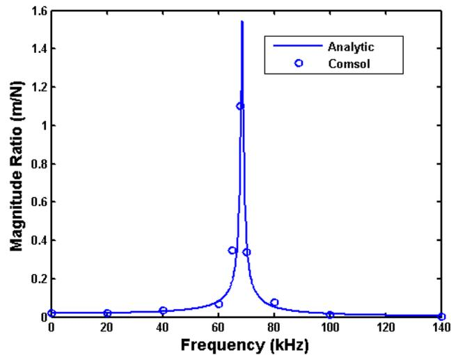
**Figure 8.** Comparison of analytical and numerical frequency responses for square plate with no hole, at ambient pressure of 300 Pa, with folded leg stiffness of 0.5165 N/m.
