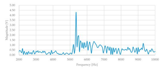
Figure 12. Out-plane frequency response of the proposed tri-axis accelerometer.
