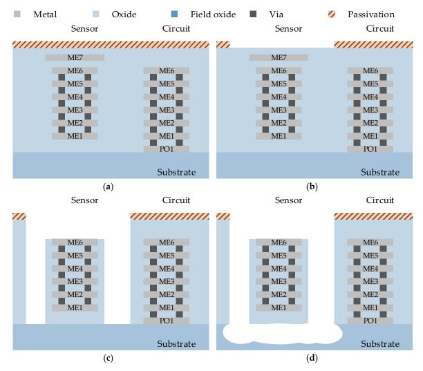
**Figure 1.** Cross-sectional view of the application-specific integrated circuit (ASIC)-compatible complementary metal-oxide semiconductor (CMOS)/micro-electromechanical system (MEMS) process flow: (a) The standard CMOS process with an additional patterned metal7 (ME7) layer; (b) The thick photoresist passivation layer is deposited for etch protection; (c) The anisotropic silicon oxide dry etching; (d) The isotropic silicon substrate dry etching.
