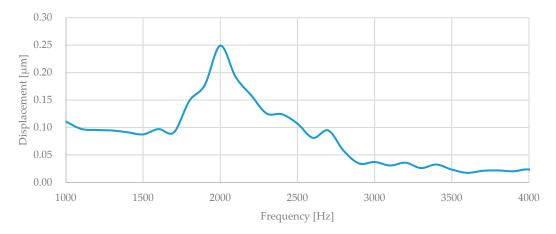
Figure 10. Frequency response of the proposed single axis accelerometer.
