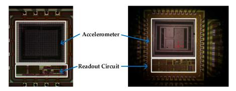
**Figure 6.** The chip die photo: (a) The single axis test chip; (b) The tri-axis test chip.
