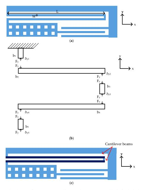
**Figure 3.** The schematic of serpentine spring: (a) Spring design parameters; (b) The free body diagram; (c) The proposed simplified model.
