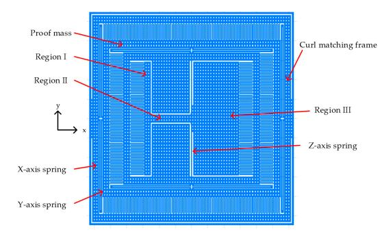
**Figure 4.** Top view of the proposed tri-axis accelerometer.
