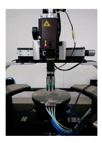
Figure 11. Measurement setup for out-plane vibration characterization.
