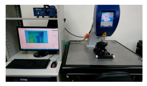
Figure 8. Measurement setup surface topography measurement.
