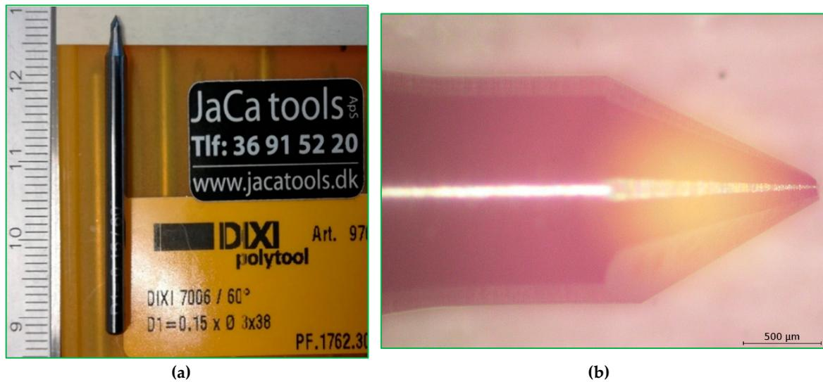
**Figure 2.** (a) Digital picture of the milling tool, DIXI 7006. (b) Microscopic picture of the tip of the milling tool (engraving tool  $\frac{3}{4}$ ).
