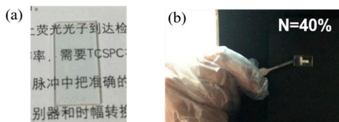
**Figure 8.** (a) The anti-counterfeiting symbol “T” on the quartz substrate. (b) The bright “T” symbol under 325 nm light irradiation.
