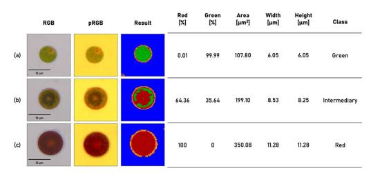
**Figure 5.** Results of multispectral data processing and spectral modeling. Microscope RGB image from reference camera (left). Processed pseudo RGB image from snapshot-mosaic camera (middle) Result image after multispectral classification (**a**) Green reference cell (**b**) Intermediary cell (**c**) Red reference cell.
