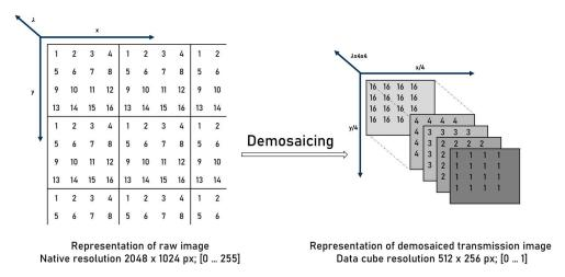
Figure 3. Resolution and value range of snapshot-mosaic camera images.
