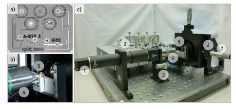
**Figure 1.** (a) Microfluidic chip with (I) Sample inlet, (II) Sheath fluid 1, (III) Sheath fluid 2, (IV) Flow Focusing Unit 1, (V) Flow rotation unit, (VI) Flow focusing unit 2, (VII) MIFC detection channel and (VIII) Waste outlet; (b) Chip integration; (c) Optical system with (1) Snapshot-mosaic camera, (2) Pressure-pump fluid management system, (3) Z-focus, (4) 20× Objective, (5) Microfluidic chip, (6) XY-linear stage, (7) LED white light source.
