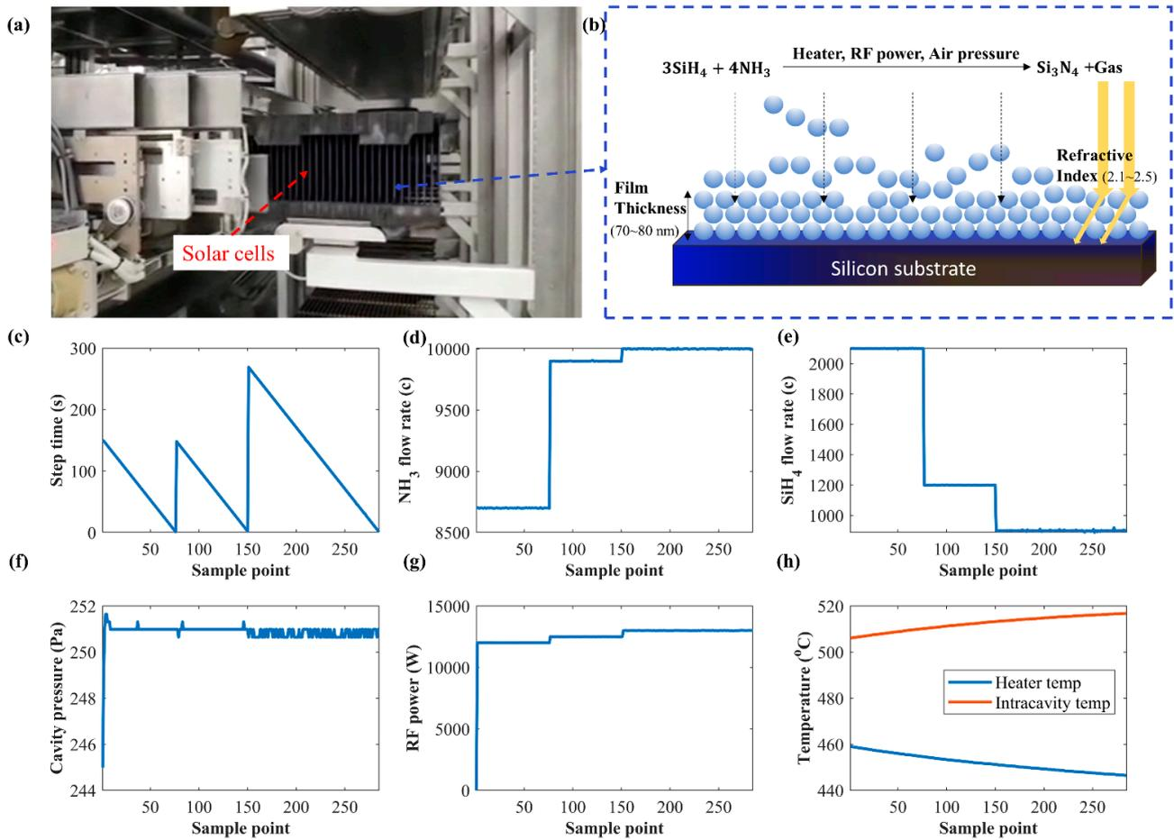
**Figure 4.** PECVD-based SiNx thin-film deposition process. (a) The real production process. (b) The schematic diagram of PECVD reaction process. (c–h) The data of control parameters collected from sensors.
