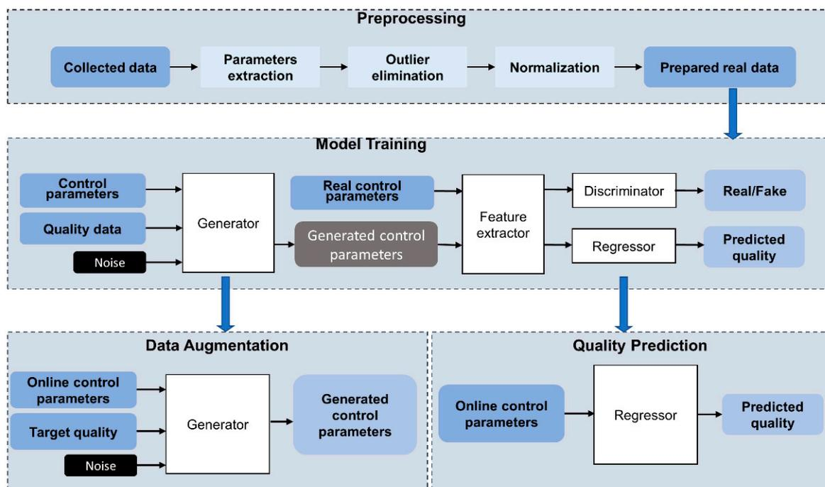
Figure 2. Overview of NCM process modeling using AR-SAGAN.
