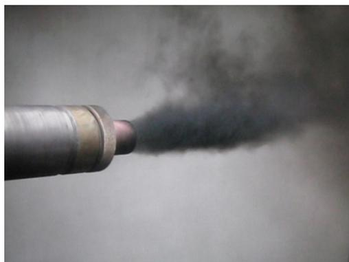
**Figure 1.** A shot of the pulse gas-detonation device (PGDD): nanoscale detonation carbon (NDC) is emitting from the barrel.
