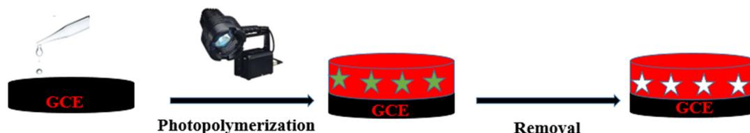
**Figure 1.** Schematic illustration of the ACR-ZDV-MIP/GCE sensor fabrication.
