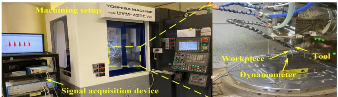
Figure 2. The hardware installation of the ultra-precision milling experiment.
