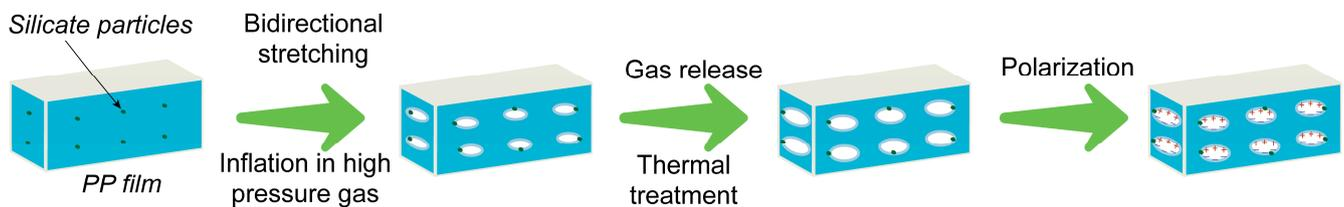
**Figure 4.** A schematic description of the processing steps of FENG.
