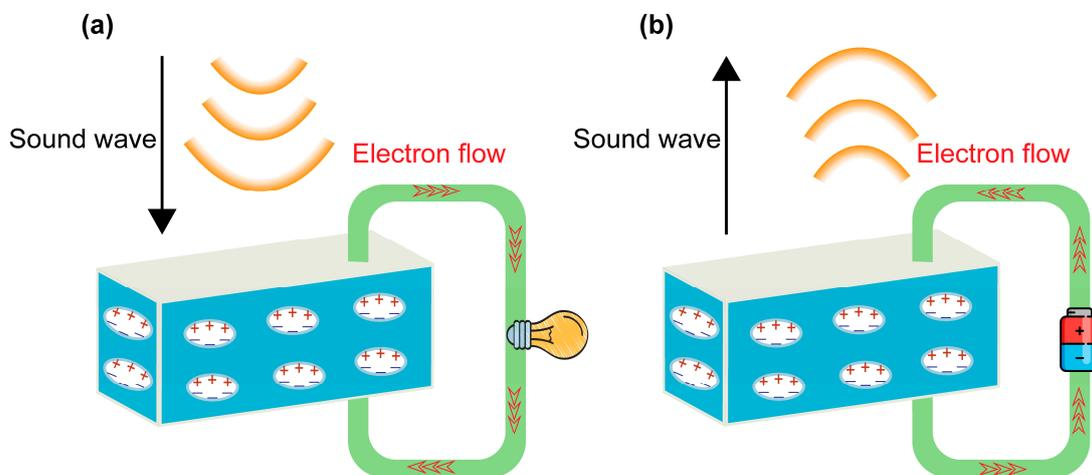
**Figure 3.** (a) The mechanism of using FENG to convert sound energy into electrical energy. (b) The mechanism of using FENG to convert electrical energy into sound energy.
