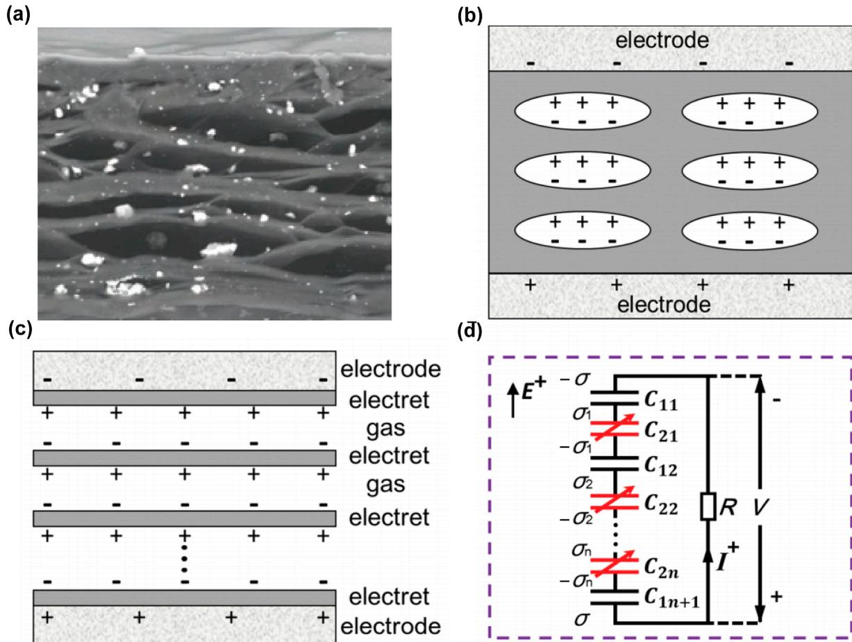
**Figure 2.** (a) Cross-sectional SEM image of a FENG based on cellular polypropylene. Reprinted with permission from Ref [17]. Copyright 2016, Elsevier BV. (b) Schematic illustration, (c) simplified structure, and (d) equivalent circuit model of a FENG. Reprinted with permission from Ref. [47]. Copyright 2016, John Wiley and Sons.
