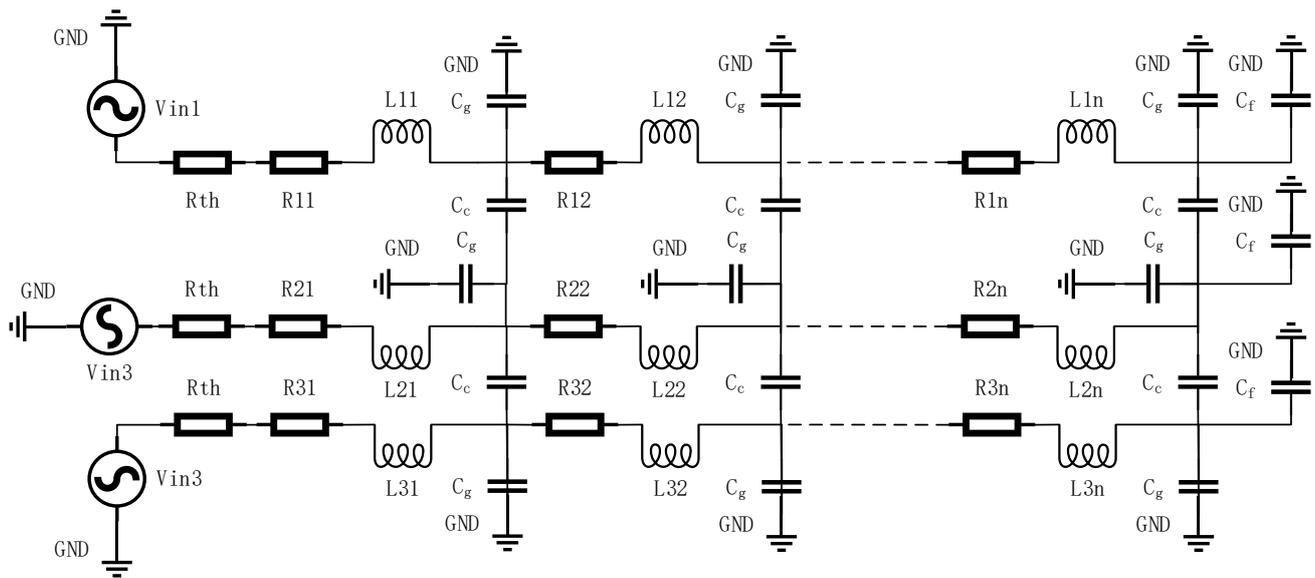
Figure 2. Distributed three-wire RLC spice model.
