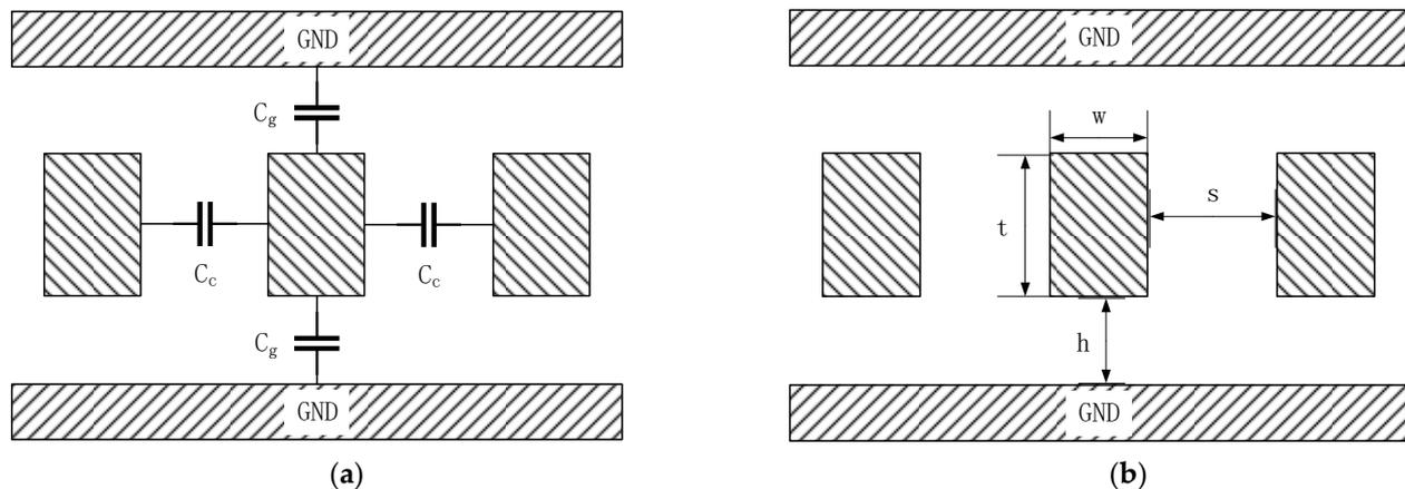
**Figure 1.** A coupling interconnect model: (a) is the equivalent capacitance model; (b) is the dimensions of an interconnect.
