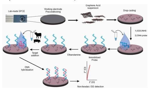
**Figure 4.** Functionalization of screen-printed carbon electrode with a graphene acid suspension to enable a specific ssDNA grafting for sensing of pork DNA using the nonfaradaic EIS. Adapted with permission from [150].
