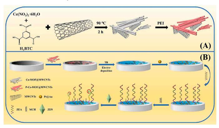
**Figure 6.** Illustration of synthesis of P-Ce-MOF@MWCNTs (**A**) and stepwise construction of the electrochemical aptasensor for trace detection of zearalenone (**B**). Adapted with permission from [96].
