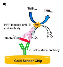
**Figure 5. (A)** Illustration of biochip integrating the microfluidics and electronic connection for biosensor. **(B)** *E. coli* detection strategy, adapted with permission from [164].
