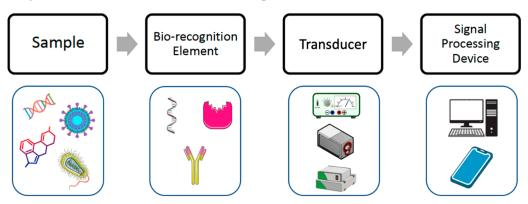
**Figure 2.** Different elements and steps in electrochemical detection of foodborne contaminants. Food sample containing biological or chemical hazardous elements in contact with the biorecognition element immobilized on the electrode generates an electrical signal that can be processed by a computer or a smartphone.
