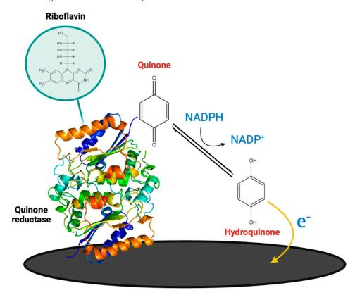
**Figure 9.** Schematic illustration of the carbon screen printed electrode modification with quinone reductase enzymatic biosensor construction and detection of vitamin  $K_3$  in solution containing NADPH as an electron donor and riboflavin.
