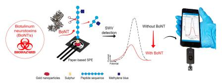
**Figure 7.** Botulinum neurotoxins detection using the peptide-based electrochemical biosensor. Thiolate peptide carrying methylene blue was grafted on AuNPs deposited onto a paper electrode. In the presence of the toxin, the peptide is cleaved, and voltammetric signal decreases. SWV, square wave voltammetry. Adapted with permission from [172].
