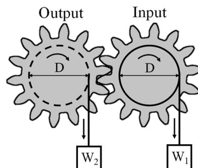
**Figure 2.** Principle of moment balance method.
