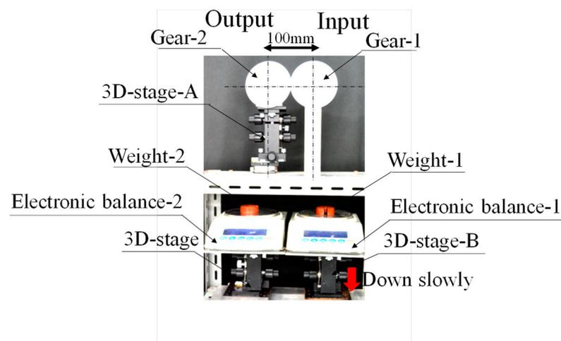
**Figure 3.** Equipment of measuring power transmission efficiency of macro gears by moment balance method.
