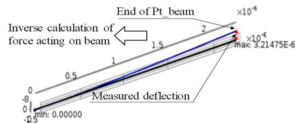
**Figure 5.** Calculation of forces using the finite element method.
