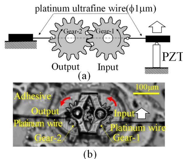
**Figure 4.** Moment balance method for micro gears. (a) Schematic of the method. (b) Real view of measurement.
