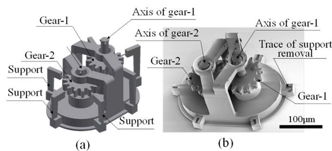
**Figure 1.** SEM image of micro-gear. (a) 3D CAD design. (b) SEM image of produced gear.
