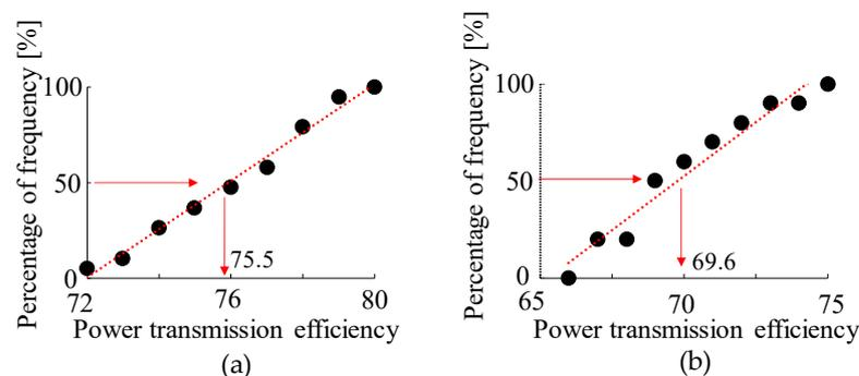
**Figure 11.** Confirmation of normality of power transmission efficiency. (a) Macro gear. (b) Micro gear.
