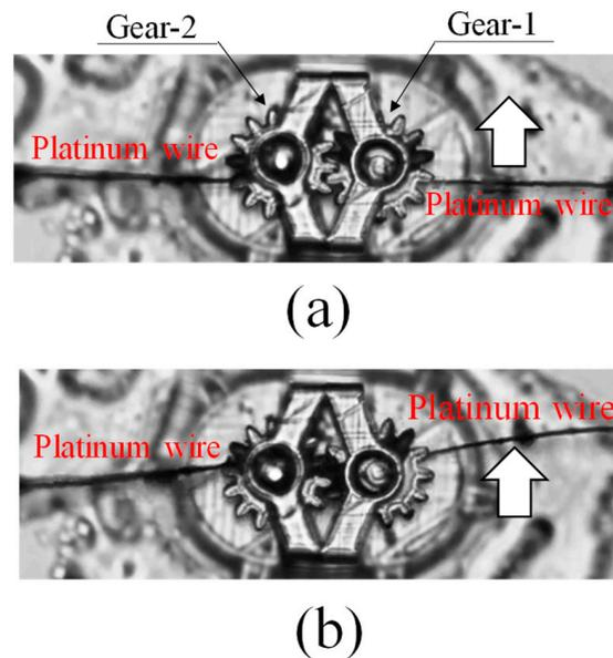
**Figure 6.** Process of measurement by moment balance method. (a) Before rotating input-micro-gear (Gear-1). (b) Rotated output-micro-gear (Gear-2).
