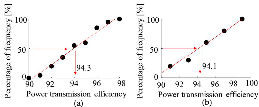
**Figure 7.** Confirmation of normality of power transmission efficiency of gears with two gears. (a) Macro gear. (b) Micro gear.
