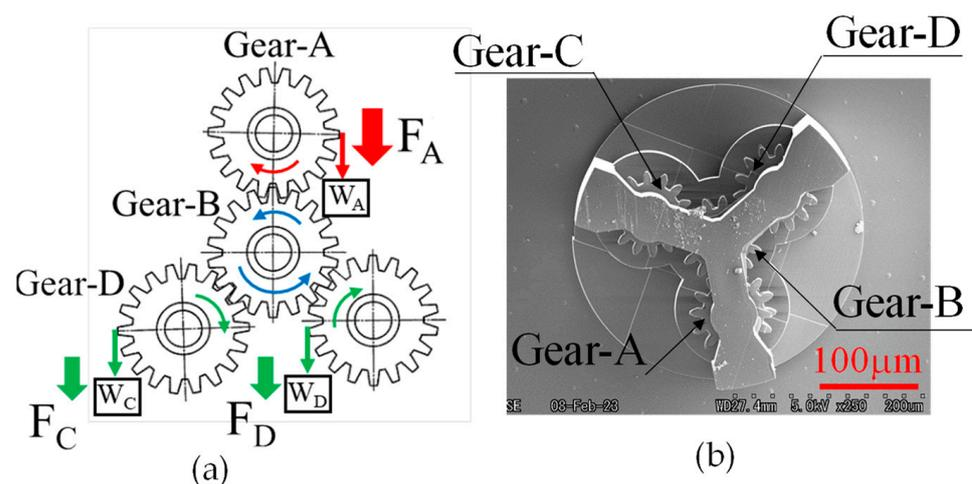
**Figure 8.** Gear train with four gears. (a) Schematic of the method. (b) SEM image of gear-train by four micro gears.
