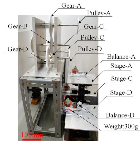
**Figure 9.** Equipment for measuring power transmission efficiency by the moment balance method in the case of four macro gears.
