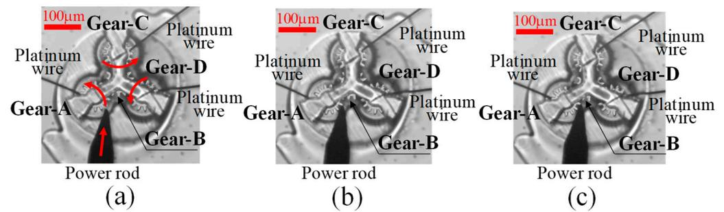
**Figure 10.** Measurement process of micro-gear train. (a) Setting of rotating micro-gear. (b) Start of rotating input-micro-gear. (c) Rotated output-micro-gear.
