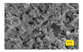
Figure 2. SEM morphology of Si<sub>3</sub>N<sub>4</sub> plate before laser processing.
