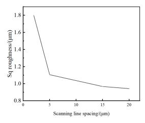
Figure 12. Roughness (Sq) versus scanning line interval.
