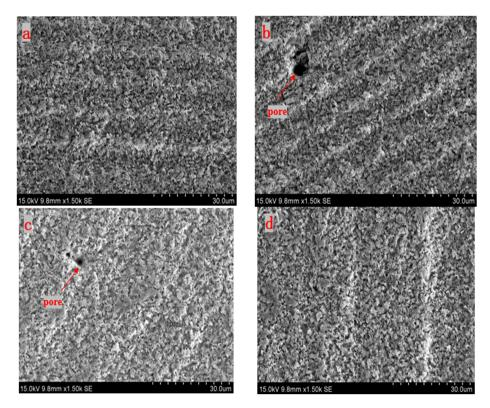
**Figure 4.** SEM images of treated surface morphologies under different scanning paths (**a**)  $\beta = 0^{\circ}$ , (**b**)  $\beta = 30^{\circ}$ , (**c**)  $\beta = 60^{\circ}$ , and (**d**)  $\beta = 90^{\circ}$ .
