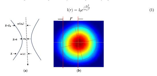
**Figure 10.** Schematic illustration of the profile and light intensity distribution of a Gaussian beam. (a) Contour of Gaussian beam. (b) Light intensity distribution on the cross-section of a Gaussian beam.
