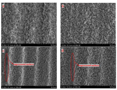
value of 1.800  $\mu m$  when the scanning line spacing is 2  $\mu m.$  The surface roughness decreases exponentially with the increase in scan line spacing.
