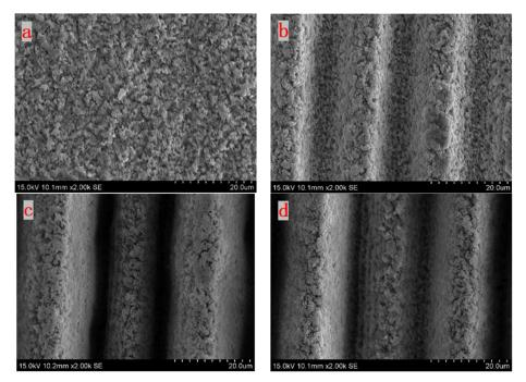
**Figure 13.** SEM image of the surface processed under different scan numbers (**a**) 1 time, (**b**) 5 times, (**c**) 15 times, and (**d**) 25 times.
