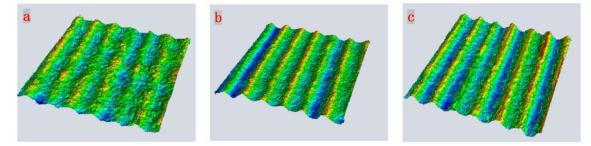
Figure 8. Three-dimensional geometric images (a) 5 µJ, (b) 20 µJ, and (c) 30 µJ.
