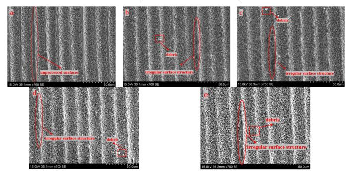
**Figure 7.** SEM images of the surface under different single energy processing (**a**) 5  $\mu$ J, (**b**) 10  $\mu$ J, (**c**) 15  $\mu$ J, (**d**) 20  $\mu$ J, and (**e**) 30  $\mu$ J.
