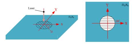
Figure 3. The laser scan path and the laser polarization direction.
