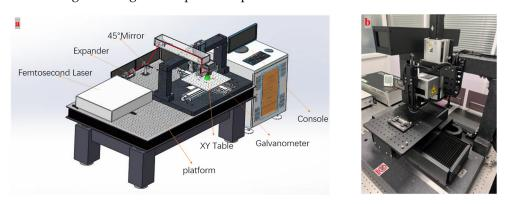
Figure 1. FemtoYL-40 Infrared femtosecond laser. (a) Integral composition. (b) Processing platform.
