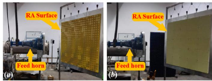
Figure 7. The experimental setups of the RA with (a) RA element I and (b) RA element II.
