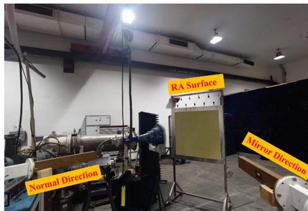
**Figure 16.** Measured setup of the directivity testing under HPM.
