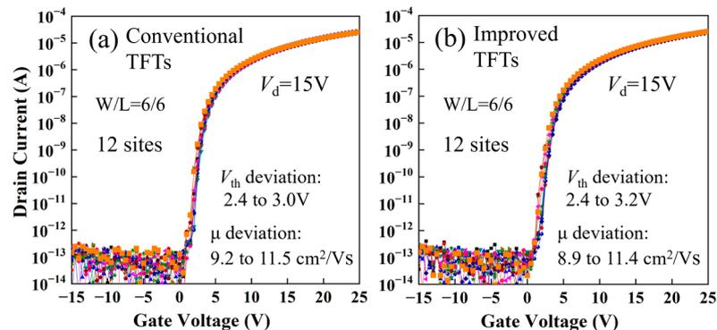
**Figure 5.** The transfer characteristics of the 12 fabricated TFTs on a G4.5 glass substrate, with (a) the conventional TFTs and (b) the improved TFTs.
