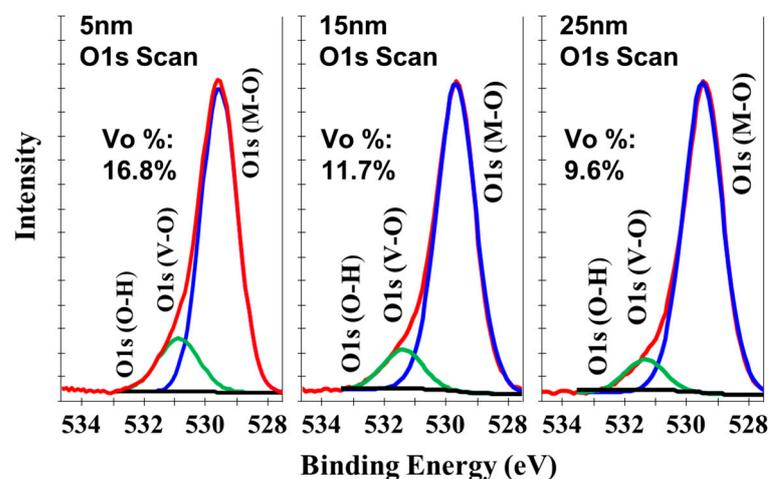
**Figure 3.** XPS spectra of the O 1s signal of a-IGZO film-4 in Table 1 at the detection depths of 5, 15 and 25 nm.
