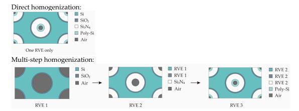
**Figure 5.** Schematic of two homogenization methods.
