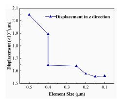
**Figure 4.** Mesh independence test by refining the mesh for the 1/4 RVE model.
