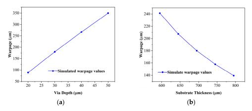
Figure 9. The effect of (a) via depth, (b) substrate thickness on wafer warpage.
