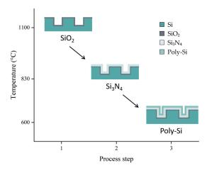
**Figure 1.** Simplified schematic of manufacturing process. Si substrate; SiO<sub>2</sub> layer deposition at  $1100 \,^{\circ}$ C; Si<sub>3</sub>N<sub>4</sub> layer deposition at  $830 \,^{\circ}$ C; Poly-Si layer deposition at  $600 \,^{\circ}$ C.
