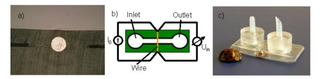
The anemometric flow sensor shown in Figure 8(c) consists of a 100  $\mu$ m high, 500  $\mu$ m wide, and 1 cm long channel from poly propylene (PP) which is crossed by a gold wire with a diameter of 50  $\mu$ m. Two 500  $\mu$ m thick PP foils were molded with a force of 100 N, ultrasonic amplitude of 9  $\mu$ m for 150 ms, 500 ms cooling time, and with an ultrasonic energy of 16 J.
