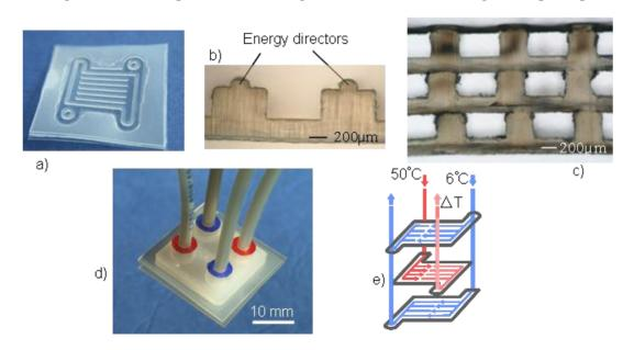
Three layers of micro grooves were welded on top of each other to build up the heat exchanger. First, the lid was welded onto the first channel layer, and then two more channel layers followed. Ultrasonic welding was performed at 60 N, 100 ms ultrasound with  $9 \text{ } \mu\text{m}$  amplitude, 500 ms cooling time, and consumed 10 J. The heat exchanger was pressurized with 200 kPa and no leakage could be observed.
