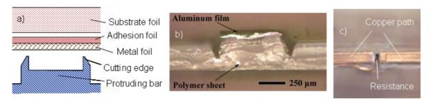
A cut through a 10 µm thick aluminum conductor path welded to a PP substrate foil, 150 µm in thickness, is shown in Figure 9(b). The width of the conductor path is 500 µm. It is clearly seen that the edge on the tool cut through the metal and adhesion foils into the substrate foil. RFID antennas and number pads for PC keyboards have been fabricated by employing this technique [17].
