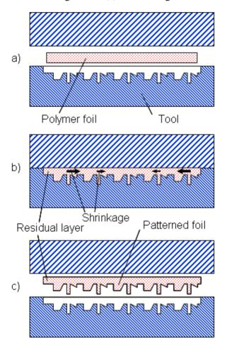
The cycle time of both injection molding and hot embossing is within the range of a few minutes, because the entire tool needs to be heated up and cooled down again. This is called a variotherm process which is required to fill all micro cavities in the mold.
