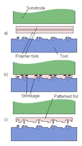
The sonotrode of an ultrasonic welding machine presses the foil or the stack of foils onto the tool and the ultrasound heats up the polymer where it is in contact with the protruding micro structures. If more than one foil is used, heat is generated not only at the interface of tool and foil but also in between the foils. Therefore, a stack of foils is warmed up from inside which enhances the melting of the polymer. Thus, less power is necessary to pattern the polymer.
