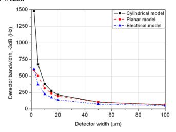
We have seen that if the detector width becomes less than 10 µm for this cavity size, the system heads toward a first order circuit response. In such a case, it will only be the gas nature (see Section 4) and the gas pressure which will condition the bandwidth of the thermal accelerometer. In the next section, the influence of this last parameter on the global sensor response will be demonstrated.
