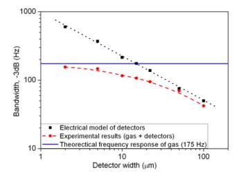
In Figure 8, the experimental response is compared to the one we obtained with the electrical model (9) assuming  $f_{c,b} = 175$  Hz, for a detector width equal to 2  $\mu$ m. We can conclude that the experimental answer is in concordance with the simulated sensor frequency bandwidth at -3 dB.
