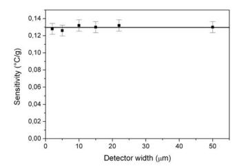
**Figure 6.** Experimental thermal sensitivity *vs.* detector width.
