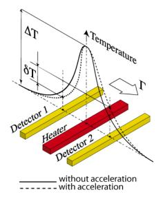
In this document, the thermal accelerometer response is theoretically evaluated and experimentally measured. Specific parameters are taken into account to design the sensor, like the size of the detectors and simple models are used for a better understanding of the thermal behavior and the frequency
