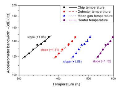
Inducing a variation of external temperatures, the gas temperature was modified, as were detectors and the heater. In each case, bandwidth was estimated and results are reported in Figure 11 as a function of the substrate, detector and heater temperatures for the experimentally obtained values, and as a function of the calculated mean gas temperature. Bandwidth, as a function of the latter, moves as  $T^{1.58}$ , value close to air thermal diffusivity behavior,  $T^{1.62}$ .
