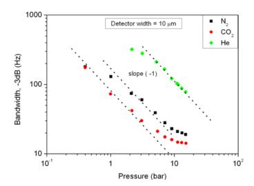
**Figure 10.** Experimental results of the sensor bandwidth at −3 dB *vs.* gas pressure.
