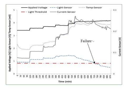
Figure 10. Sensor data from accelerated life test.
