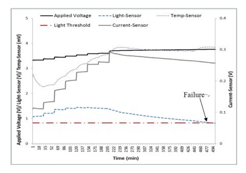
Figure 13. Sensor data from accelerated life test.
