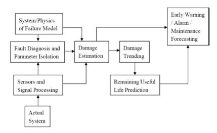
**Figure 2.** Block diagram of a model driven approach.
