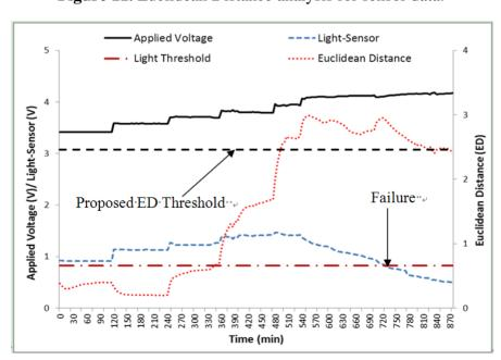
Figure 11. Euclidean Distance analysis for sensor data.
