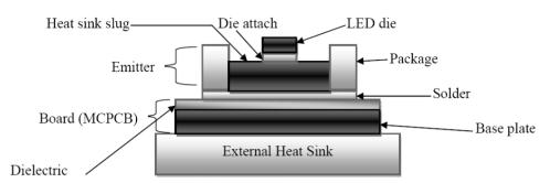
**Figure 5.** Cross section of LED assembly.
