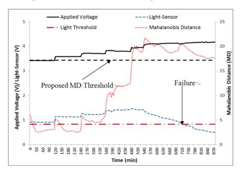
Figure 12. Mahalanobis Distance analysis for sensor data.
