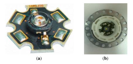
Figure 7 details the experimental test setup, which consists of a data acquisition system (National Instruments PXI), a voltage regulator and sensors, and a single High Power Philips Luxeon Star LED. For purpose of light measurement the LED is placed within a semi spherical enclosure which also contains a photodiode light sensor.
