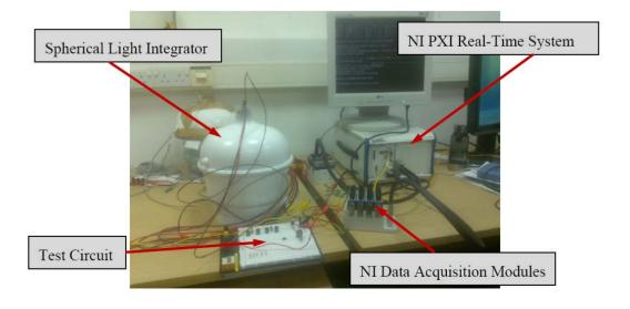
The National Instruments PXI platform can be connected to both analog and digital input modules providing the ability to measure voltage levels for different types of signals. For this experiment we use a 24-bit universal analog input module (NI 9219) to measure the applied voltage, and the voltage across the three sensors (current, temperature, and light).
