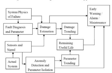
Figure 3. Block diagram of a fusion approach.
