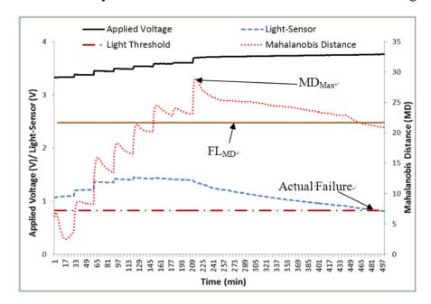
**Figure 17.** MD history and the MD failure limit for LED test data in the Figure 13.
