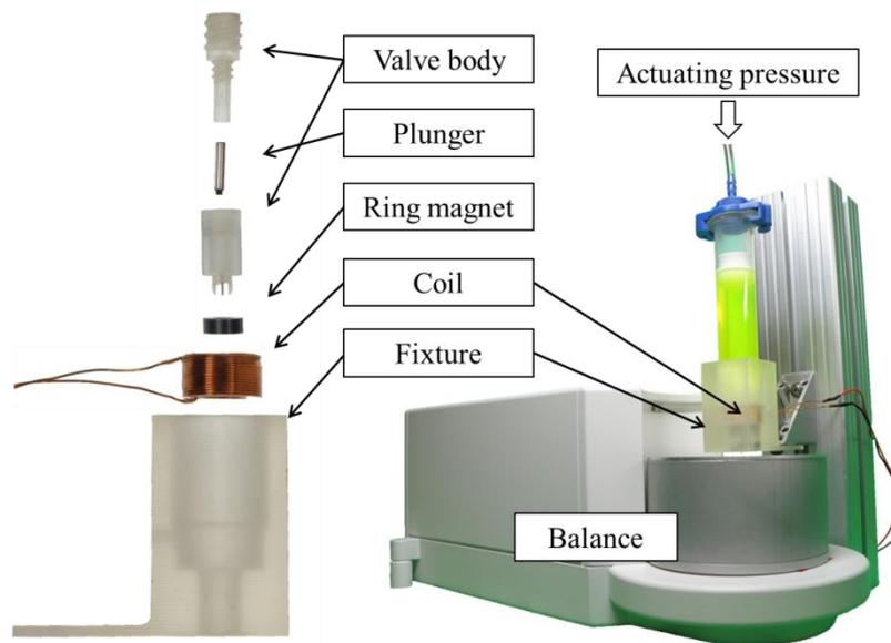
The dispensing performance has been characterized with water ( $\eta = 1.03$  mPas) and 66% (w/w) glycerol/water solution ( $\eta = 16.98$  mPas). The pressure was set to 200–400 mbar for water and 800 mbar for glycerol to compensate for the higher viscosity.
