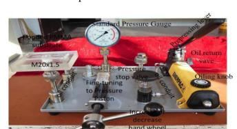
Figure 5. The burst test setup connected with the bonded PMMA substrate.
