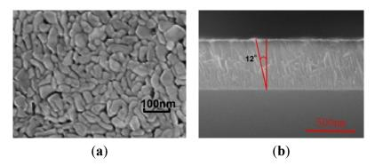
Figure 1. (a) The surface morphology of AlN film; and (b) The cross-section of sample.
