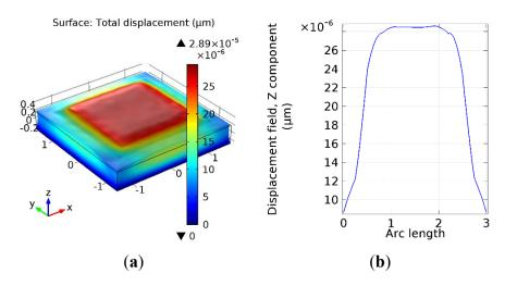
**Figure 5.** The simulation results for the sample with a top electrode; (**a**) a three-dimensional figure of the surface deformation and (**b**) the *z*-axis displacement along the center line at 7 V.
