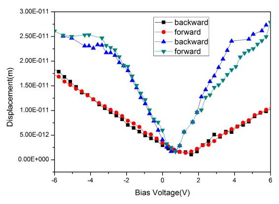
**Figure 8.** The piezoelectric strain curves obtained in the measurement; the black and red curves are for the sample without a top electrode, and the green and blue curves are for the sample with a top electrode.
