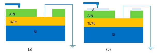
Figure 3. The testing schematics of the experimental samples, (a) the sample without the top electrode and (b) the sample with the top electrode.
