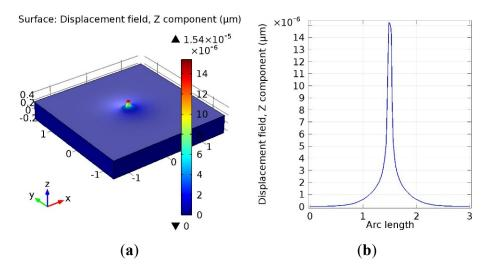
Figure 4. The simulation results for the sample without a top electrode; (a) a three-dimensional figure of the surface deformation and (b) the *z*-axis displacement along the center line at 7 V.
