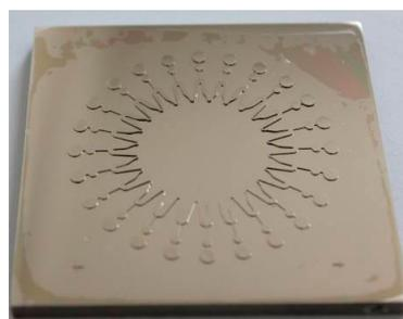
**Figure 9.** The microfluidic chip mold.
