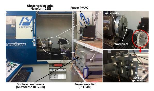
Figure 5. Machine setup of cutting experiments.
