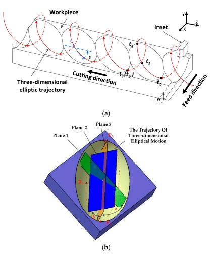
**Figure 1.** Principle of the non-resonant three-dimensional elliptical vibration cutting (3D-EVC) technique. (a) Cutting process of the non-resonant three-dimensional elliptical vibration cutting (3D-EVC); (b) Individual cutting marks in a single cutting cycle.
