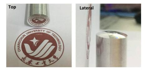
**Figure 11.** Convex spherical surface topography of titanium alloy machined by a non-resonant three-dimensional elliptical vibration cutting (3D-EVC) apparatus ( $f_{3D} = 50 \text{ mm/min}$ , S = 50 mm/min,  $A = 7 \mu\text{m}$ ,  $D = 1 \mu\text{m}$  and  $F = 0.2 \text{ mm/min}^{-1}$ ). (**left**) Top view; (**right**) Lateral view.
