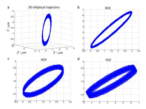
**Figure 4.** Tool trajectory of non-resonant three-dimensional elliptical vibration cutting (3D-EVC).  $A_1 = 7 \ \mu m$ ,  $A_2 = A_3 = 4 \ \mu m$ ,  $\phi_1 = 0$ ,  $\phi_2 = \pi/2$ ,  $\phi_3 = \pi$ ,  $\omega_1 = \omega_2 = \omega_3 = 50 \ \text{Hz}$ . (a) The spatial elliptical trajectory; (b) The projection of the 3D elliptical trajectory in the XOZ plane; (c) The projection of 3D elliptical trajectory in the XOY plane; (d) The projection of the 3D elliptical trajectory in the YOZ plane.
