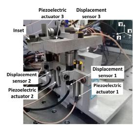
**Figure 2.** Apparatus of the non-resonant three-dimensional elliptical vibration cutting (3D-EVC) in cutting experiments.
