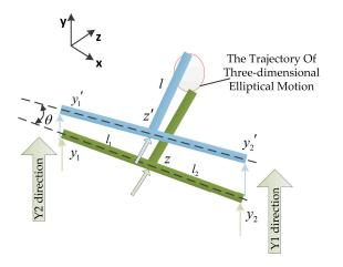
Figure 3. The generation principle of three-dimensional elliptical motion in the tool tip.
