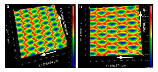
**Figure 9.** Effect of vibration frequency on surface topography machined by non-resonant three-dimensional elliptical vibration cutting (3D-EVC) apparatus ( $S = 50 \text{ mm/min}, A = 7 \mu \text{m}, D = 1 \mu \text{m}$  and  $F = 0.2 \text{ mm} \cdot \text{min}^{-1}$ ). (a) The vibration frequency in the tool tip was  $f_{3D} = 50 \text{ Hz}$ ; (b) The vibration frequency in the tool tip was  $f_{3D} = 30 \text{ Hz}$ .
