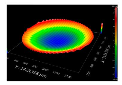
**Figure 10.** Concave spherical surface topography of titanium alloy machined by a non-resonant three-dimensional elliptical vibration cutting (3D-EVC) apparatus. ( $f_{3D} = 50 \text{ mm/min}$ , S = 50 mm/min,  $A = 7 \mu\text{m}$ ,  $D = 1 \mu\text{m}$  and  $F = 0.2 \text{ mm} \cdot \text{min}^{-1}$ ).
