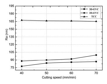
**Figure 7.** Surface roughness under different cutting speeds. ( $f_{2D} = f_{3D} = 50$  Hz,  $A = 7 \mu m$ ,  $D = 1 \mu m$  and  $F = 0.2 \text{ mm} \cdot \text{min}^{-1}$ ).
