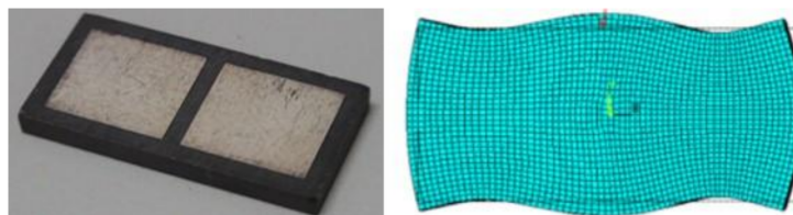
Figure 2. (a) The used piezoelectric material and (b) deformation simulation of the used piezoelectric material.
