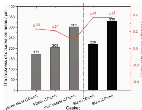
**Figure 4.** Gasket category and thickness with the corresponding thickness of the PDMS observation area.
