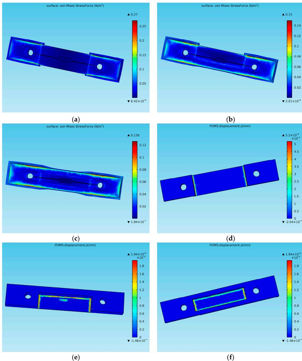
**Figure 5.** The simulation diagram of the stress and deformation in the z-direction of three kinds of PDMS replica structures in bonding process. Stress of bottom surface of: (a) Replica A; (b) Replica B; and (c) Replica C. Deformation in the z-direction of: (d) Replica A; (e) Replica B; and (f) Replica C.
