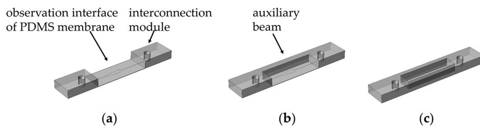
**Figure 2.** Three kinds of PDMS replicas structures with observation interface of PDMS membrane: (a) Replica A without auxiliary beam; (b) Replica B with one auxiliary beam; (c) Replica B with two auxiliary beams.
