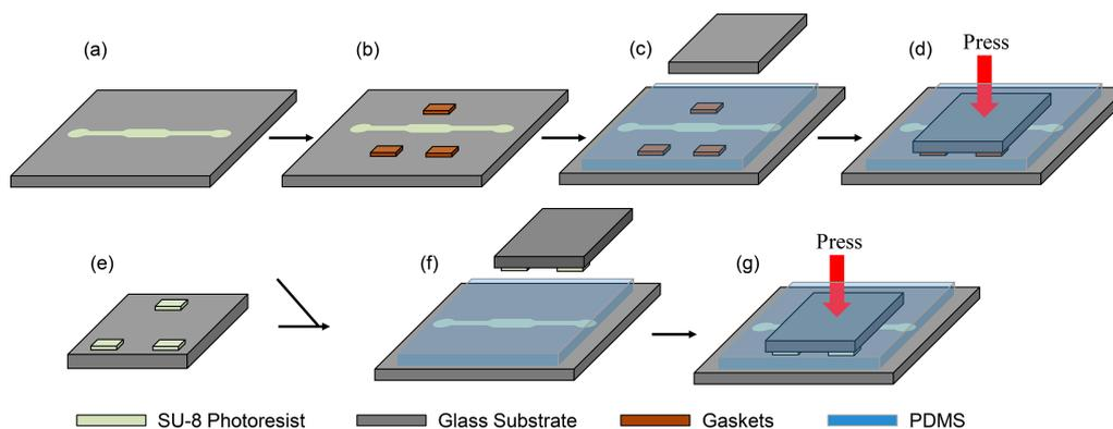
**Figure 3.** The scheme illustration of the two kinds of fabrication process of one-step molding: (a–d) the first process with silicon, polyvinyl chloride (PVC) and PDMS gaskets; (e,f) the second process with SU-8 gaskets. (a) microfluidic channel of SU-8; (b) gasket placement around the channel; (c) PDMS casting; (d) placement of the cover glass; (e) SU-8 gaskets; (f) PDMS casting; and (g) placement of the SU-8 glass wafer.
