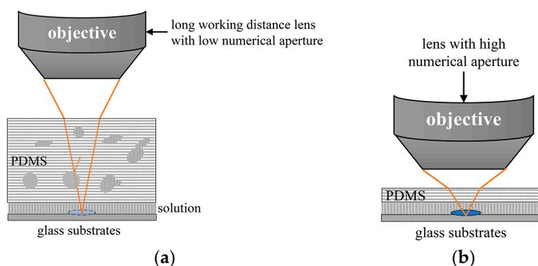
**Figure 1.** The scheme illustration of microscopic examinations: (a) observation of the particles in thick polydimethylsiloxane (PDMS)-based microfluidics; (b) observation of the particles in PDMS-based microfluidics with thin observation interface via the objective of high numerical aperture.
