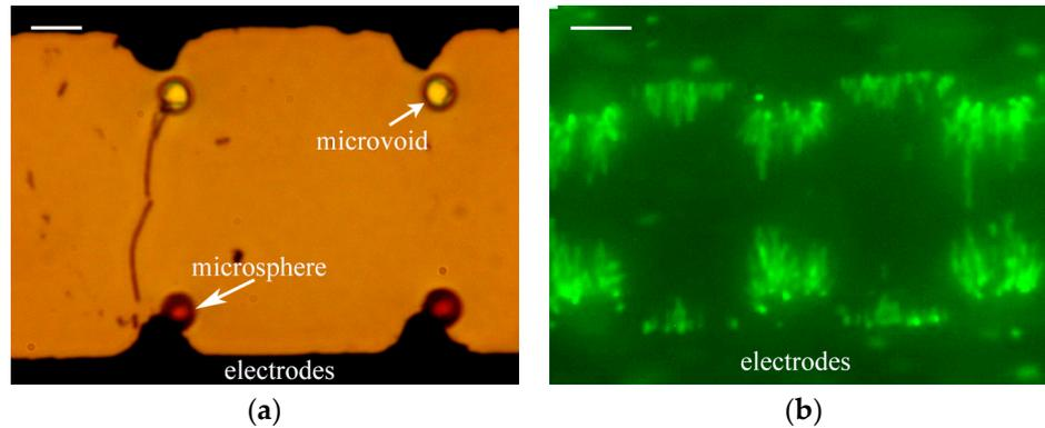
**Figure 7.** Photographs of two kinds of dielectrophoresis microfluidics chips with thin observation interfaces: (a) optical images of red trapped polystyrene (PS) microspheres in microfluidic chip, scale bar: 5  $\mu\text{m}$ ; and (b) fluorescence images of trapped bacteria in microfluidic chip, scale bar: 10  $\mu\text{m}$ .
