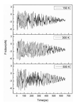
Figure 6. Variation of friction force between shells with time for temperatures of 150, 300, and 500 K.
