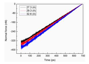
Figure 4. Variation of normal force between shells with time for three outer shell diameters.
