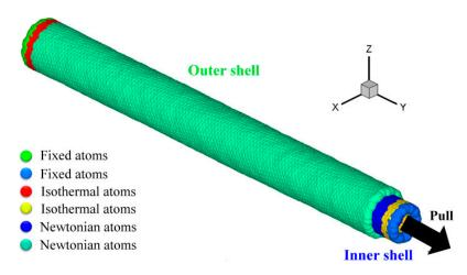
**Figure 1.** Molecular dynamics (MD) model of double-walled carbon nanotubes (DWCNTs). The model consists of an inner shell and an outer shell, whose lengths are both 30 nm. The diameters of the outer and inner shells are 2.73 and 2.4 nm, respectively.
