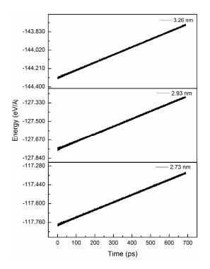
Figure 5. Variation of interaction energy with time for three outer shell diameters.
