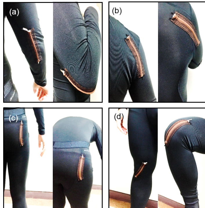
Figure 9. Flexion and extension motions at the four positions of (a) elbow; (b) shoulder; (c) hip, and (d) knee on application of the maximum bending condition.
