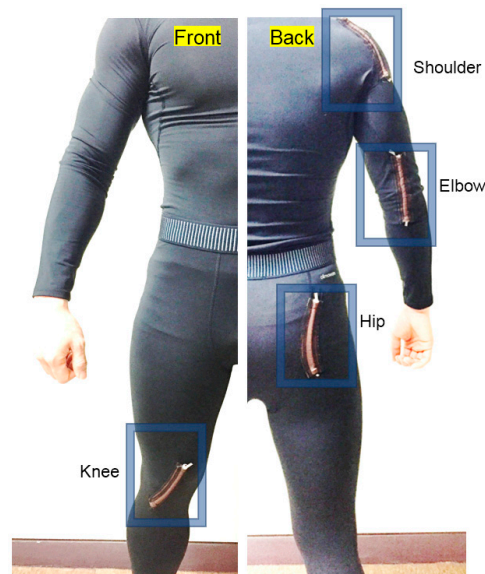
Figure 5. Photographs of the front (left) and back (right) views of the wearable energy harvesting garments.
