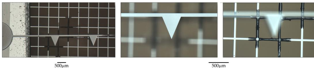
**Figure 11.** A typical failure mode of an electrode set. Permanent damage is sometimes observed following sparkover from a wire tip to the collector grid. This may be due to the relatively high current density following dielectric breakdown causing rapid Joule heating in the grid wires, or due to physical ablation during the high current breakdown. After a destructive event such as this, both electrodes were replaced despite there being no visible damage to the emitter wire.
