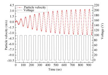
Figure 2. The particle velocity and its corresponding pulse voltage.
