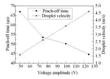
Figure 6. The pinch-off time and droplet velocity varies with different amplitudes of pulse voltages.
