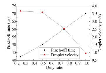
Figure 9. The pinch-off time and droplet velocity vary with different duty ratios.
