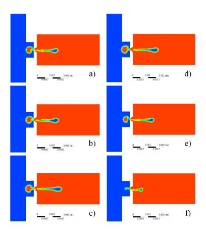
**Figure 11.** The injection status varies with different duty ratios: (a)  $\alpha = 0.25$ ; (b)  $\alpha = 0.35$ ; (c)  $\alpha = 0.5$ ; (d)  $\alpha = 0.6$ ; (e)  $\alpha = 0.75$ ; (f)  $\alpha = 0.99$ .
