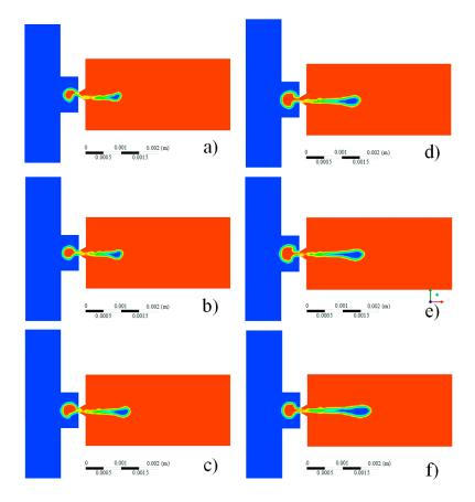
**Figure 8.** The injection status varies with different voltage amplitudes: (**a**) 50 V; (**b**) 60 V; (**c**) 75 V; (**d**) 90 V; (**e**) 100 V; (**f**) 125 V.
