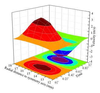
Figure 3. The velocities of the particles in the fluid-solid coupling interface.
