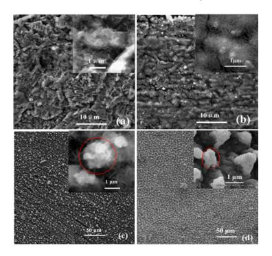
**Figure 2.** SEM images of nano-structures prepared at 70 °C in acidic solution for (**a**) 5 min; (**b**) 20 min, and (**c**) 30 min; (**d**) SEM image of the lotus leaf surface [35].
