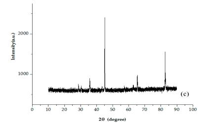
**Figure 3.** EDS spectrum of the carbon steel ball surface before (**a**) and after (**b**) oxidation; (**c**) XRD pattern of the oxidation nanosheet. Red boxes represent diffraction peaks of  $Fe_3O_4$ .
