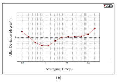
**Figure 8.** (a) Input-output characteristic of the proposed rotational gyroscope; (b) Log-log plot of ADEV versus the averaging time for the angular speed of the proposed rotational gyroscope.
