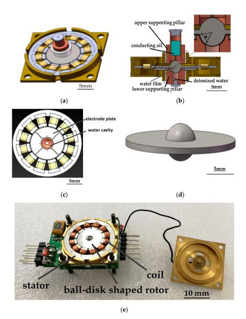
**Figure 1.** (a) Gyroscope structure assembly diagram without the upper frame; (b) Assembly cross-section diagram; (c) Engineering diagram of the electrode plate and water cavity; (d) Engineering diagram of the ball-disk-shaped rotor; (e) Photo of the fabricated gyroscope.
