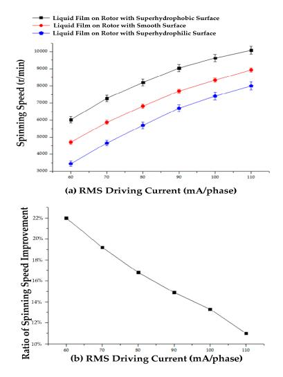
**Figure 6.** (a) Steady-state spinning speed under different RMS driving currents; (b) The ratio of the spinning speed improvement compared between rotor with smooth and superhydrophobic surfaces under different RMS driving currents.
