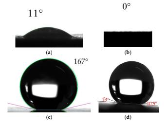
**Figure 4.** Optical photo of water droplets on surfaces with different morphology: (a) untreated sheet surface; (b) sheet surface after oxidation; and (c) superhydrophobic sheet surface; (d) Snapshot photograph of the advancing CA and receding CA of the superhydrophobic sheet surface.
