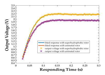
**Figure 7.** Fitted curve of the output voltage under the step angular speed input of 20°/s for gyroscopes with and without a superhydrophobic rotor.
