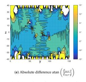
**Figure 7.** Difference between the dielectrophoretic force computed with COMSOL software according to the parameters given in Figure 5 and the one computed with Matlab according to the analytical model proposed in this paper. (**a**,**b**) give the relative difference in percentage and (**c**,**d**) give the absolute difference on the dielectrophoretic force in Newton along both the  $\vec{y}$  and  $\vec{z}$  axes. (**e**) gives the error on the force orientation in degrees.
