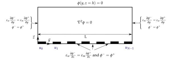
**Figure 2.** Schematic representation of the boundary conditions determining the electric potential above an array of electrodes.  $\phi^+$  and  $\phi^-$  are the electric potentials on each side of the boundary.  $\varepsilon_m$  is the permittivity of the fluid in the channel and  $\varepsilon_w$  is the permittivity of the wall.
