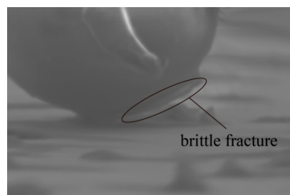
Figure 6. Photo exhibiting brittle fracture of the adherent interface formed between the sphere-substrate interface.
