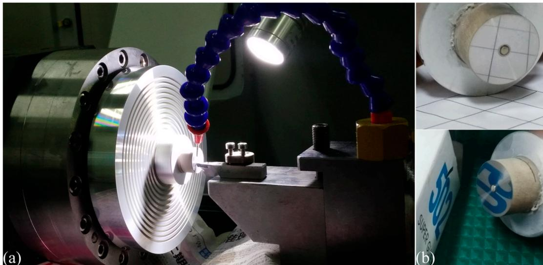
**Figure 10.** (a) Configuration of diamond cutting of cerium; (b) machined surface of cerium at the DOC of 5  $\mu\text{m}$ .
