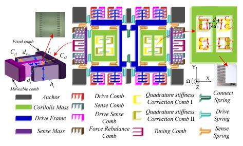
Figure 1. Mechanical model of dual-mass MEMS gyroscope.
