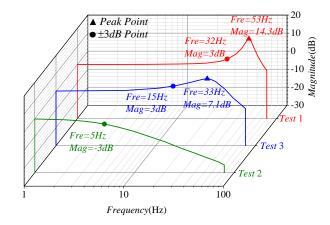
Figure 16. Gyroscope bandwidth under the three test methods.
