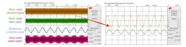
Figure 13. The test curves of the frequency tuning system.
