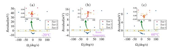
**Figure 15.** The residual errors of the scale factor under different temperatures: (**a**) -20 °C condition, (**b**) Room temperature condition, (**c**) 60 °C condition.
