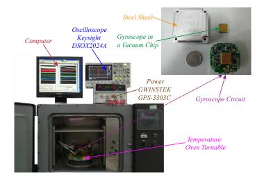
Figure 12. Photos of the MEMS gyroscope circuit and test equipment.
