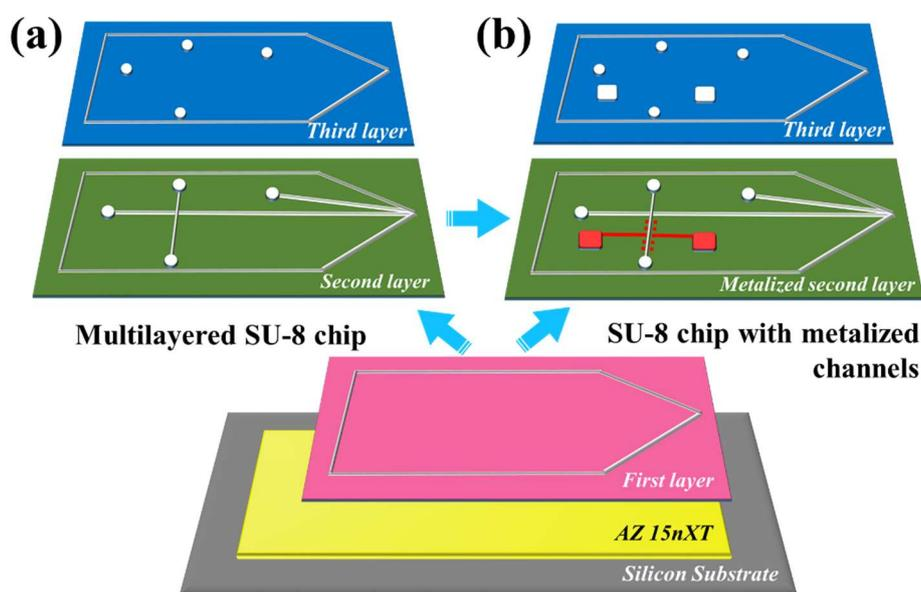
**Figure 1.** Schematics of multilayer SU-8 free-standing microfluidic device for mass spectroscopy electro spray ionization. (a) the multilayered SU-8 ESI chip (b) SU-8 chip with extra metallization step.
