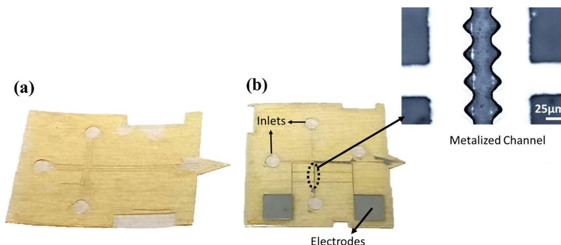
**Figure 2.** Microfabricated multilayer SU-8 chips (a) the multilayered SU-8 electro spray ionization (ESI) chip for mass spectrometer analysis (b) metalized SU-8 chip with electrodes. The insert shows the channels which are metalized by lift-off.
