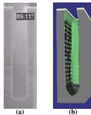
Figure 8. The SEM photography (a), and the simulation result (b) of a single trench.
