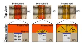
**Figure 2.** Hydrogen ion diffusion experiment (**top row**) and cross-section schematic (**bottom row**) using the 3D-printed cross-channel diffusion chip. The phenol red in the channel (t = 0 s) gradually changed to yellow at the channel intersection (t = 10 s) until it turned completely yellow (t = 70 s), while the bottom channel did not change color.
