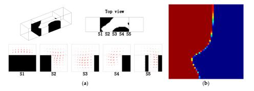
**Figure 6.** (a) Layout of the micromixer for the design domain as shown in Figure 4, where n = 2, Re = 5, and projected velocity vector distribution in the cross sections (S1, S2, S3, S4, S5); the mixing measurement  $J_{C_0}(C) = 0.9147$ ; (b) the distribution of coarse grain concentration on the outlet.
