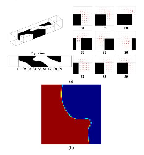
**Figure 7.** (a) Layout of the micromixer for the design domain as shown in Figure 4, where n = 4, Re = 5, and projected velocity vector distribution in the cross sections (S1, S2, S3, S4, S5, S6, S7, S8, S9); the mixing measurement  $J_{C_0}(C) = 0.8382$ ; (b) the distribution of coarse grain concentration on the outlet.
