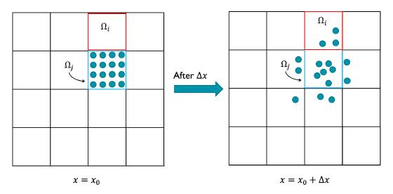
**Figure 1.** The calculation of the mapping coefficient  $\Phi_{ij}$  in the mapping matrix is the ratio of the number of markers received by the recipient cell  $\Omega_i$  at  $X = X_0 + \Delta X$  to the initial number of markers in  $\Omega_j$  at  $X = X_0$  (in this example  $\Phi_{ij} = 3/16$ ) [26,27].
