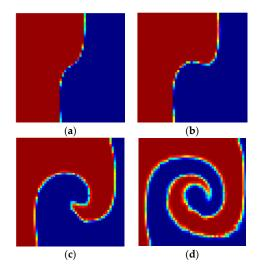
**Figure 8.** The evolution of mixing performance of micromixers with different cycles which the single cycle is the layout in Figure 5: (**a**–**d**) are the distribution of coarse grain concentration on the outlet with 1, 2, 5, and 10 cycles, and  $J_{\overline{C}}(C)$  are 0.9882, 0.9779, 0.9404 and 0.8413, respectively.
