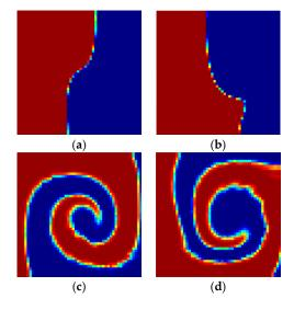
**Figure 9.** (**a**,**c**) are the distribution of coarse grain concentration on the outlet with 1 and 10 cycles shown in Figure 8a and d, and  $J_{\overline{C}}(C)$  are 0.9882 and 0.8413; (**b**,**d**) are the distribution of coarse grain concentration on the outlet of SHM (Figure 10) with 1 and 10 cycles, and  $J_{\overline{C}}(C)$  are 0.9883 and 0.8446.
