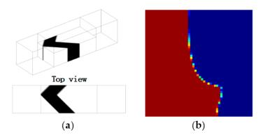
**Figure 10.** (a) Layout of the SHM in the design domain as shown in Figure 4, where n = 2, Re = 2.5, and the mixing measurement  $J_{\overline{C}}(C) = 0.9883$ ; (b) the distribution of coarse grain concentration on the outlet. (the SHM has only one groove and is same volume as the micromixer shown in Figure 5).
