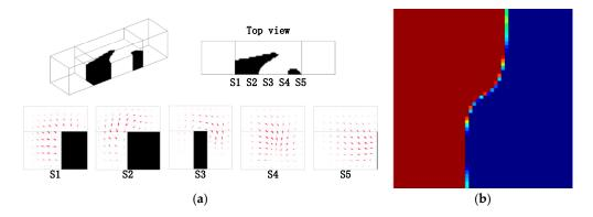
**Figure 5.** (a) Layout of the micromixer for the design domain as shown in Figure 4, where n = 2, Re = 2.5, and projected velocity vector distribution in the cross sections (S1, S2, S3, S4, S5); the mixing measurement  $J_{C_0}(C) = 0.9141$ ; (b) the distribution of coarse grain concentration on the outlet.
