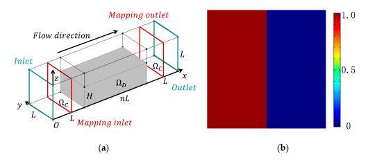
**Figure 4.** (a) Design domain  $\Omega_D$  of the micromixers at the bottom layer of the straight channel.  $\Omega_C$  is the channels connected to the inlet, outlet and design domain  $\Omega_D$ . The length of design domain  $\Omega_D$  is *n* times of *L*; (b) the distribution of coarse grain concentration on the outlet.
