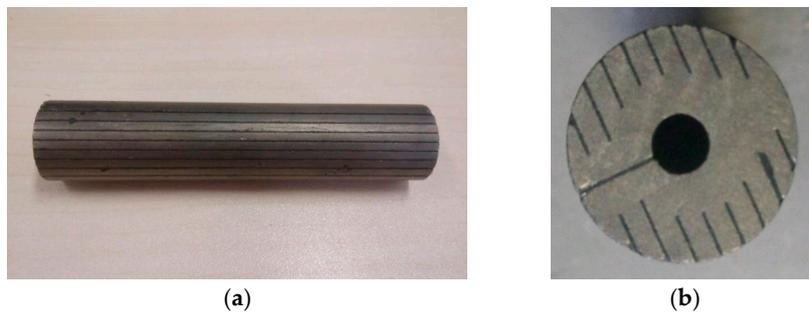
**Figure 2.** Terfenol-D rod after section treatment. (a) Terfenol-D rod; and, (b) Section treatment.
