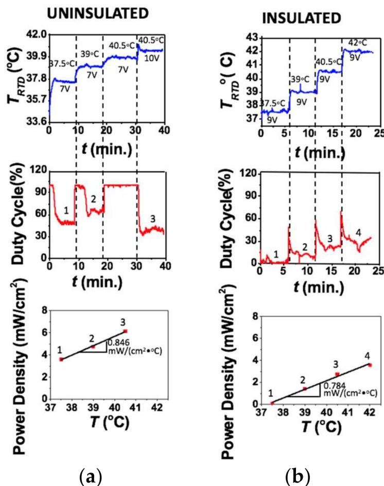
**Figure 6.** (a) Plot of heater temperature versus time as the set points and voltages are changed, followed by a plot of the corresponding duty cycle versus time. The average of the steady state duty cycles marked 1, 2 and 3 were used to calculate the power densities plotted below marked 1, 2 and 3, respectively, at different temperatures; (b) The same plots as figure A except the heater is insulated with a piece of foam.
