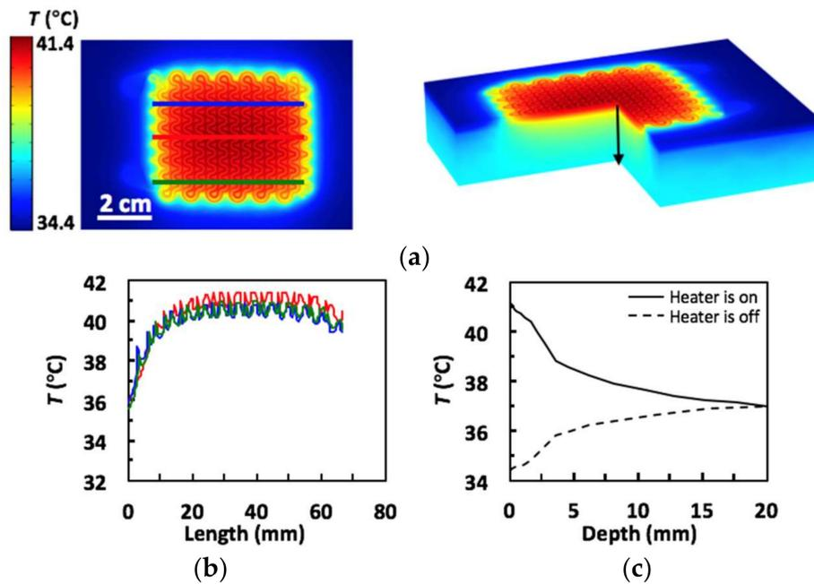
**Figure 4.** (a) COMSOL thermal simulation results (left: top view; right: 3D view); (b) Lateral heat distribution of heater. Blue, red and green lines on simulation image (left) mark the horizontal line across which temperature was collected for their respective red, blue and green plots; (c) Vertical heat distribution of skin from the black line on simulation image (right).
