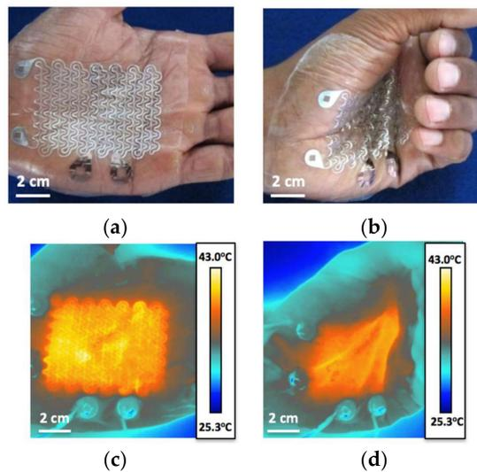
**Figure 2.** (a,b) Device conforms to hand and maintains its conformability during opening and closing; (c,d) Infrared (IR) images of the device powered with proportional-integral-derivative (PID) control as the hand is opened and closed. The PID controller automatically adjusts power output so the hand does not overheat when it closes.
