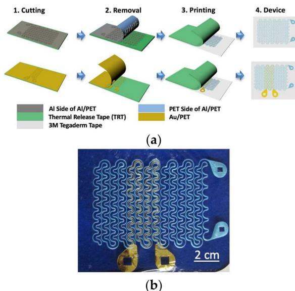
**Figure 1.** (a) Fabrication process used for heater and resistance temperature detector (RTD), shown for heater. Material is put on the thermal release tape (TRT) and cut with Silhouette cutter. TRT is heated, excess material is removed and remaining material is transferred to Tegaderm; (b) Complete device on tegaderm. Aluminum with blue polyimide backing forms the resistive heating element while Au/Cr 100/10 nm forms the resistance temperature detector.
