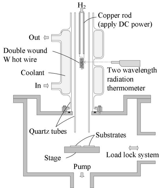
Figure 1. Schematic of the remote-type hot-wire tool.
