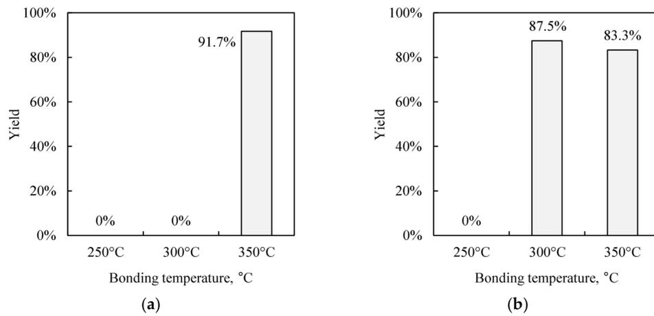
**Figure 5.** Yields of the hermetic sealed cavities. A pair of bonding wafers is exposed to the atmosphere for 1 h after each pre-treatment. (a) Citric acid treated wafer. (b) Atomic hydrogen treated wafer.
