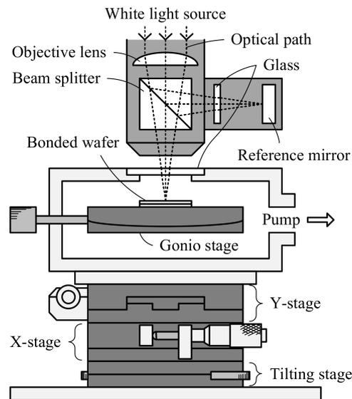
**Figure 3.** Schematic of the sealed cavity pressure evaluation by zero-balance method.
