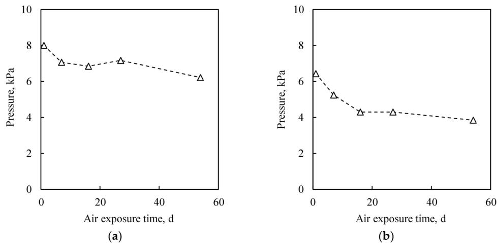
**Figure 8.** Cavity pressure change with air exposure time. (a) Citric acid treated wafer, which was bonded at 350 °C. (b) Atomic hydrogen treated wafer, which was bonded at 300 °C.
