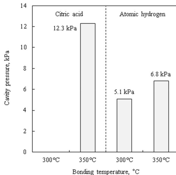
**Figure 7.** Hermetic sealed cavities pressure measured by zero-balance method.
