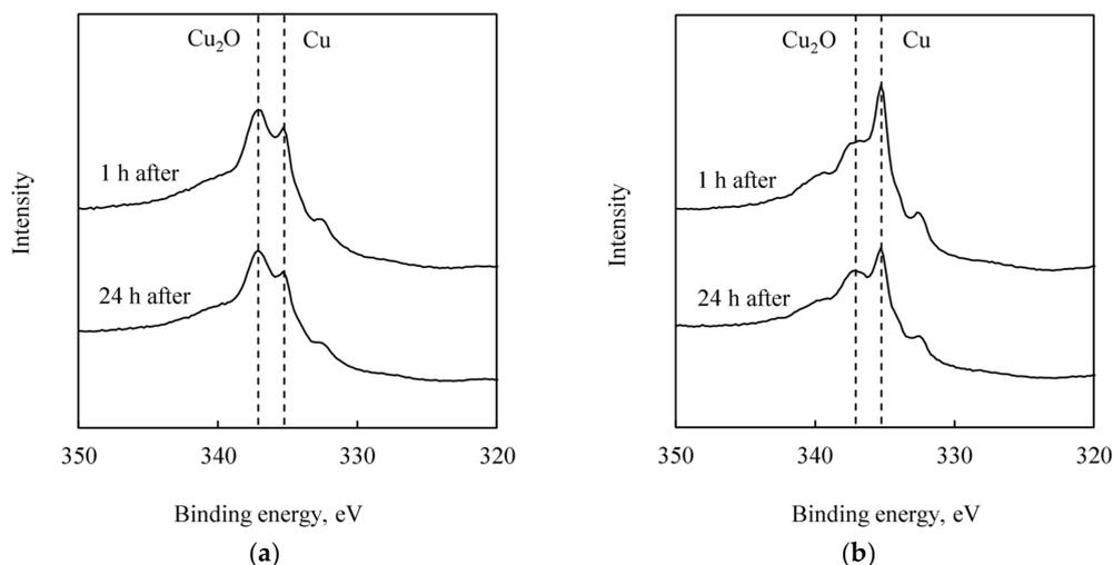
**Figure 9.** AES spectra of the treated Cu films after exposed to the air for 1 or 24 h. (a) Citric acid treated Cu film. (b) Atomic hydrogen treated Cu film.
