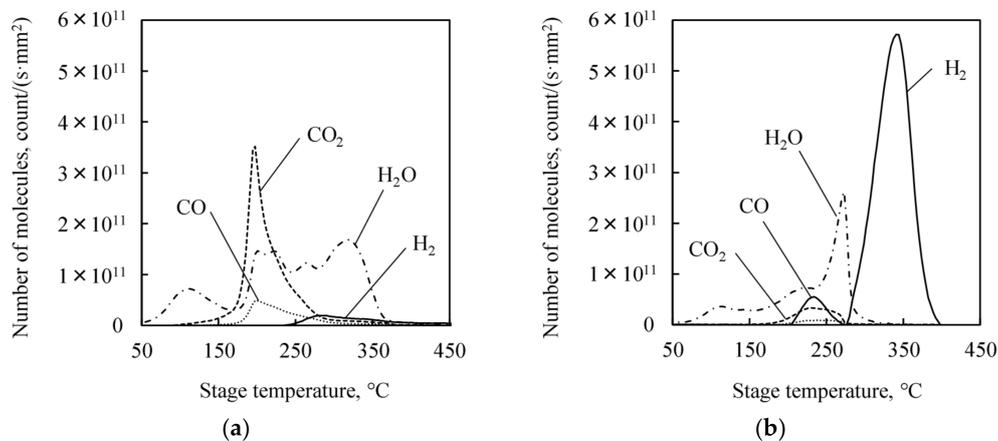
**Figure 10.** TDS spectra of the treated Cu films after exposed to the atmosphere for 1 h. (a) Citric acid treated Cu film. (b) Atomic hydrogen treated Cu film.
