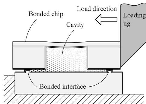
**Figure 4.** Schematic of bonding shear strength evaluation.
