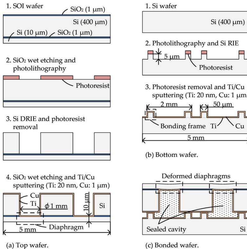
Figure 2. Fabrication processes of (a) the top wafer (cavity wafer), (b) the bottom wafer (bonding frame wafer) and (c) bonded wafer. Both wafer size is 2 cm square. Each wafer has 16 cavities with diaphragms and bonding frames.
