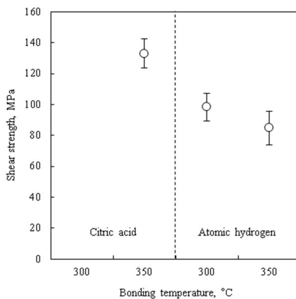
**Figure 6.** Shear strengths of the bonded chips.
