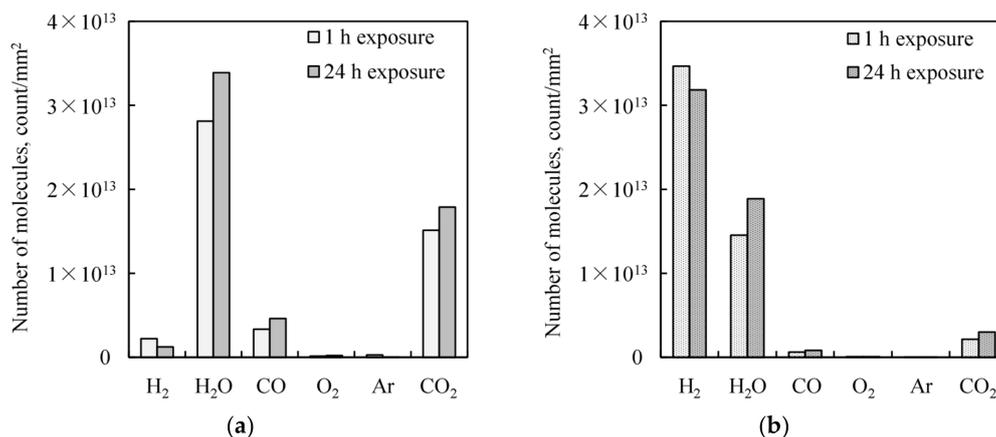
**Figure 11.** Total amounts of desorbed molecules in the TDS measurements. The treated Cu films are exposed to the atmosphere for 1 or 24 h. (a) Citric acid treated Cu film. (b) Atomic hydrogen treated Cu film.
