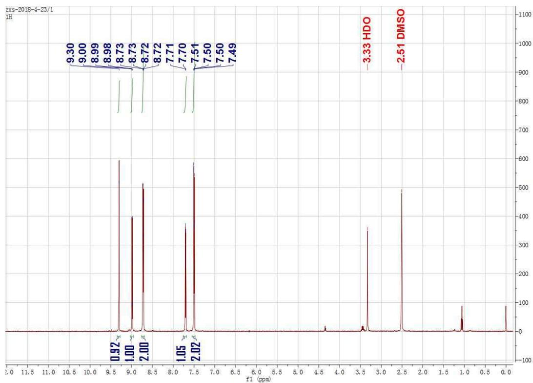
Figure S1. <sup>1</sup>H NMR spectra of 3-nitro-4,4'-bipyridine.
