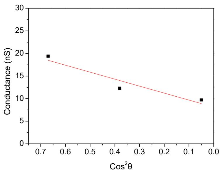
**Figure S3.** Conductance pyridine-based molecules of BPY, BPY-N and BPY-2N vs.  $\text{cos}^2\theta$ , here  $\theta$  is the twist angle between two rings.
