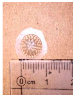
Figure 11. The sample of a bionic compound eye with a radius of 9 mm.
