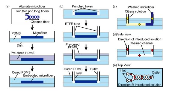
Figure 3. Process flow of the fabrication of chained PDMS microchannels. (a) Embedding of a microfiber with structure that two thin and long fibers are connected to a chained fiber into the PDMS substrate;(b) fabrication of inlets and an outlet for the microchannel; (c) removing the embedded microfiber;(d) side view of the formed microchannel; (e) top view of the formed microchannel.
