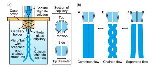
**Figure 1.** Schematic of the formation of alginate microfibers: (**a**) formation of alginate microfibers with branched structures using a theta-glass capillary; (**b**) conceptual illustrations of three flow regimes of two streams extruded from the theta-glass capillary (A: combined flow, B: chained flow, C: separated flow).
