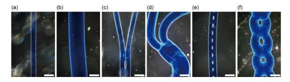
**Figure 6.** Alginate microfibers with various shapes: (**a**,**b**) single-threaded fibers formed in a combined flow regime (**a**) I and (**b**) II; (**c**,**d**) branched fibers formed in flow regimes changing from (**c**) combined flow regime I to separated flow regime I, and (**d**) combined flow regime II to separated flow regime II; (**e**,**f**) Chained fibers formed in chained flow regime (**e**) I and (**f**) II. Scale bars are 500 μm.
