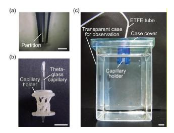
**Figure 2.** Experimental setups for alginate microfiber formation: (**a**) sharpened theta-glass capillary; (**b**) capillary holder assembled with the sharpened theta-glass capillary; (**c**) experimental setup for formation of alginate microfibers. Scale bars are: (**a**) 200 µm and (**b**,**c**) 5 mm.
