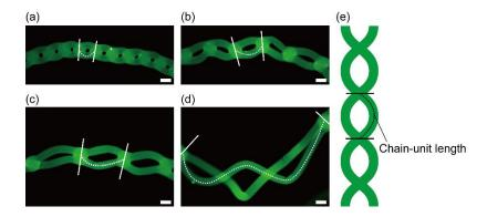
**Figure 7.** Fluorescent images of chained alginate microfibers with different chain-unit lengths. Microfibers were formed at flow rates of (**a**) 7.0 mL/min; (**b**) 7.5 mL/min; (**c**) 8.0 mL/min; and (**d**) 8.5 mL/min. The dotted line between two lines represents the chain-unit length; (**e**) Conceptual image of chain-unit lengths. Scale bars are 500  $\mu$ m.
