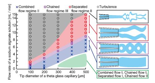
**Figure 5.** Experimental phases showing relationships between the flow regimes, flow rate of the sodium alginate solution, and tip diameter of the theta-glass capillary. Refer to Figure S1 for detailed data of the bottom-right regime.
