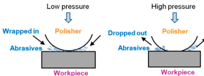
Figure 10. A general model of the material removal mechanism in vibration-assisted polishing.
