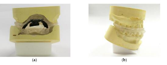
**Figure 8.** (a) Posterior view of the maxilla and mandible molds with the proposed device attached. (b) Side view of the molds with the proposed device attached.
