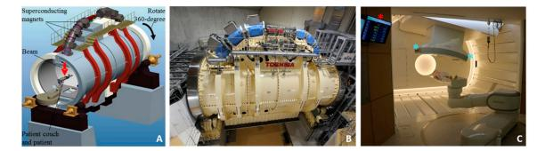
**Figure 4.** (A) Schematic diagram of the actual gantry seen in (B). Superconducting magnets, beam nozzle, and patient location are labelled. (C) A photograph showing a phantom patient on the robotic couch with the gantry in a slightly titled position. Also seen in the picture: the computer-based patient positioning system coordinates (red asterisk) and the flat panel detectors (blue asterisks).
