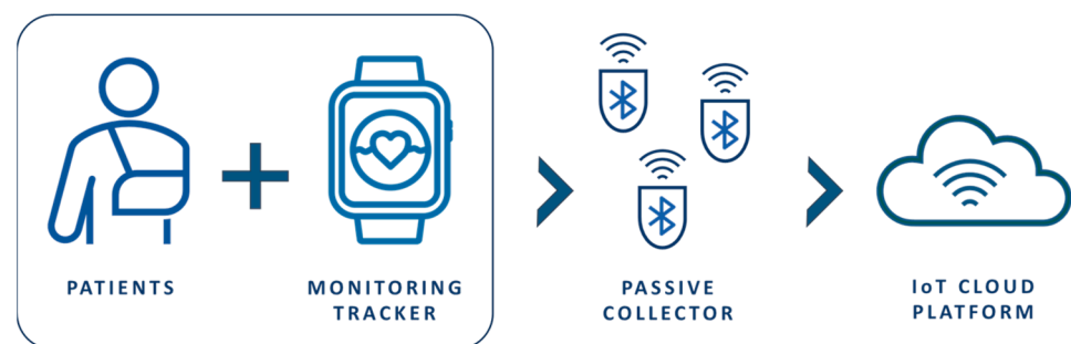
Figure 3. On-site monitoring architecture.
